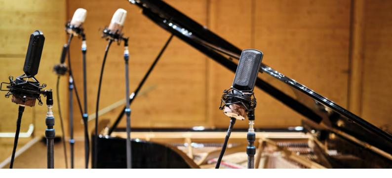
THE MICROPHONES. While in the past we mostly used only two microphones, we today can use up to 8. From 2019 on we use our own state-of-the-art ribbon microphones. The motors come from Bumblebee and Rode, the wooden housing is built by us and the output transformer is made to spec by the best transformer maker: Audio Consulting.
