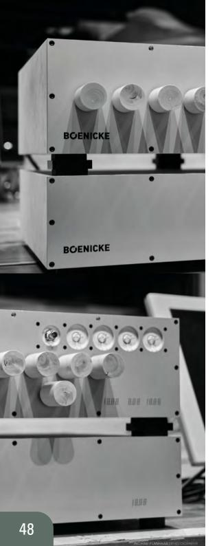
THE 8-CHANNEL MICROPHONE PREAMPLIFIER / A/D CONVERTER is a custom and handmade design by Swiss Audio Consulting (www.audio-consulting.ch). No single capacitor is used in the signal path throughout the whole design. The amplifying circuit is considered as one of the most transparent and fastest on the planet, using a minimum amount of parts, and those parts are simply the fanciest available: For example, all 8 channels together use 64 resistors only, but each one costs us 35f.
